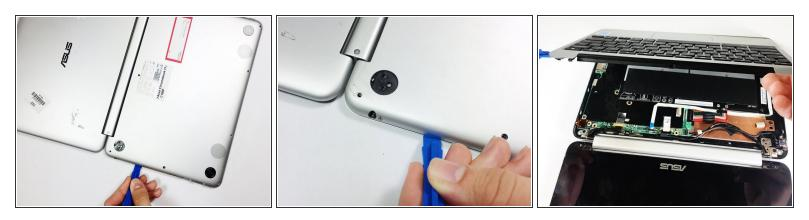
• Pry the palm rest assembly apart from the bottom cover using a spudger. This step may require a bit of elbow grease. Once the palm rest has been separated from the bottom cover, pull it away from the screen, rather than away from yourself.
