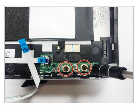
Unscrew two 2.7 mm screws using the Phillips #0 screwdriver.
