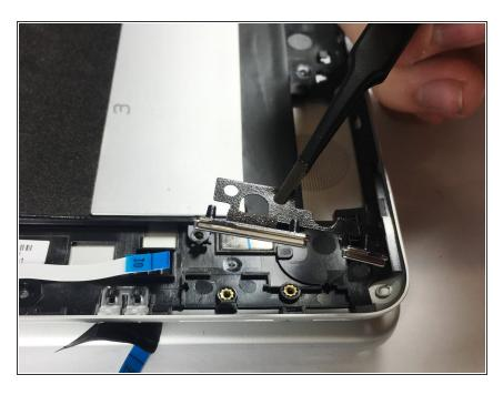
• Using tweezers, carefully pull out the external buttons.
