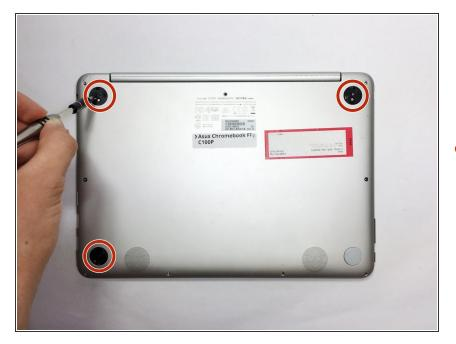
Remove the five screws from beneath the rubber feet using a philips head screwdriver. The first 1.9mm screw is located under the front right foot, the second 1.9mm screw and third 2.3mm screw are located under the rear right foot, and the fourth and fifth 2.3mm screws are located under the rear left foot.
