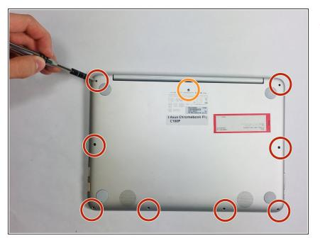
Remove the eight 3mm bottom cover screws and one 6mm screw using a T5 screwdriver. Set apart the screw in the rear middle of the bottom cover from the the other eight screws, as it is longer than them.
