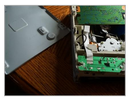
Check for any remaining screws around the edge of the board, if there are none apparent double check the ribbons and the slide the board back until it slides free
