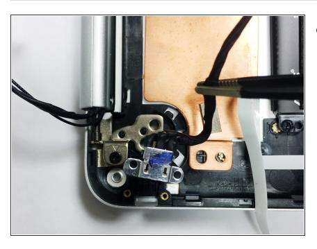
Using a pair of tweezers or your fingers, lift up the charging cable and remove the charging port.
