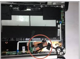
Disconnect the DC jack cable and the battery cable from the motherboard using tweezers, the pointed end of a plastic spudger, or by simply pulling the cables apart from the motherboard with your fingers.
