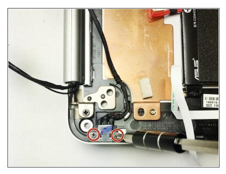
Remove the two 2.7mm screws using the Phillips #0 screwdriver.
