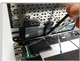
Disconnect the touchpad cable and the keyboard cable on the palm rest assembly from the motherboard using the pointed end of a plastic spudger.
