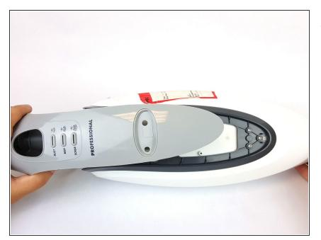
Pop off the grey front plate to expose the control panel and screws necessary to open mop body.
