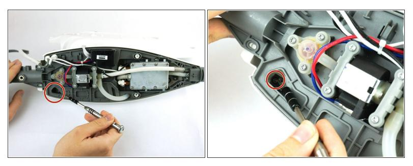
Remove the top left 12.0 mm Phillips head #2 screw from inside body.
