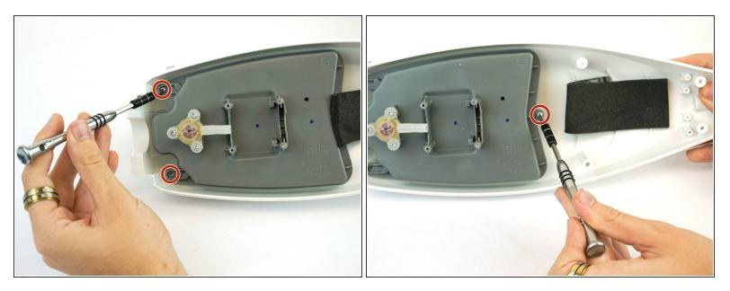
Remove two 12.0 mm Phillips head #2 screws on the top and then pull back the black foam to reveal and remove the third 12.0 mm Phillips head #2 screw.
