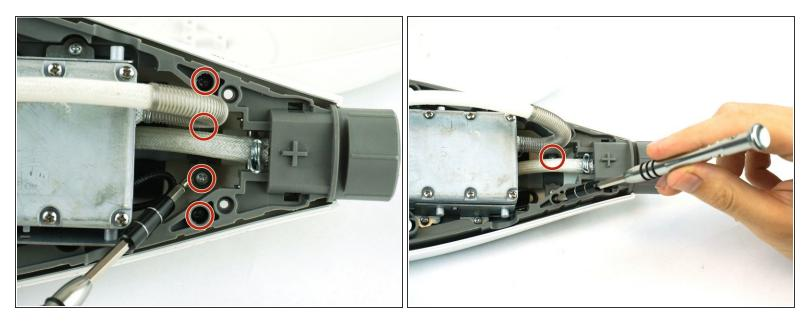
• Remove four 12.0 mm Phillips head #2 screws from the inside of the mop body.
