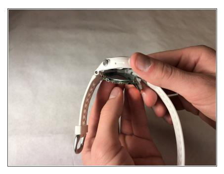
Remove the screen and motherboard assembly from the case.
