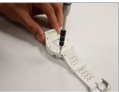
Remove the six T5 Torx 6.32mm screws securing the back cover to the watch.
