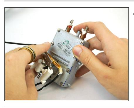
Pull apart wire connectors to fully detach the heating element.
