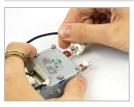
Grip each wire at its base and pull to disconnect them from the heating element.
