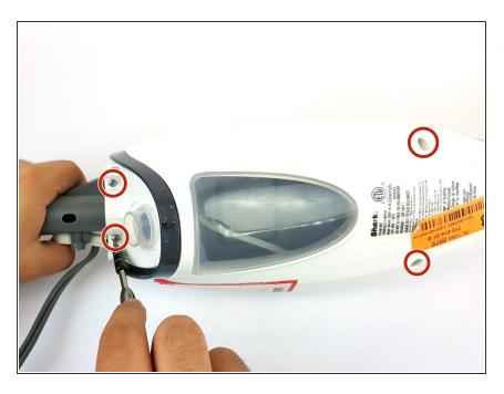
Remove the four 16.0 mm T10 Torx screws located on the back of the mop.
