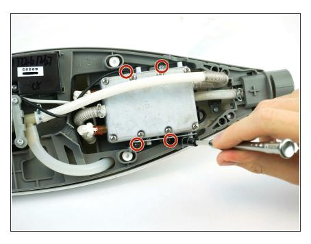
Remove the four 12.0 mm Phillips head #2 screws on the sides of the heating element.
