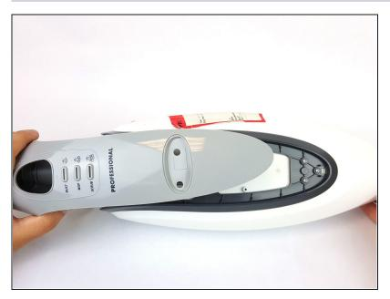
Pop off the grey front plate to expose the control panel and screws necessary to open mop body.
