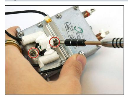
Remove two 12.0 mm Phillips head #2 screws from the heating element.
