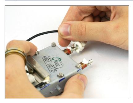
Grip each wire at its base and pull to disconnect them from the heating element.
