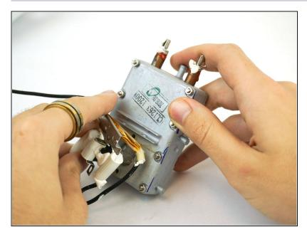
Pull apart wire connectors to fully detach the heating element.
