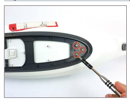
Remove the three 12.0 mm Philips head #2 screws connected to the dark grey plastic trim.
