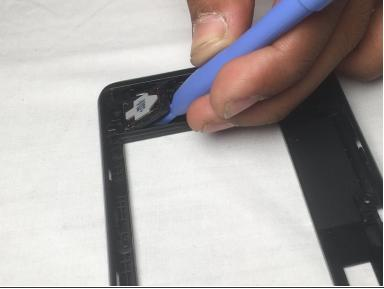
Pry the loud speaker out of the mid-frame with a plastic opening tool.
