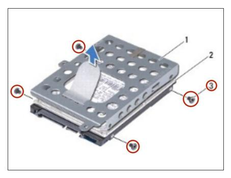
Remove the four screws that secure the hard-drive bracket to the hard drive.
