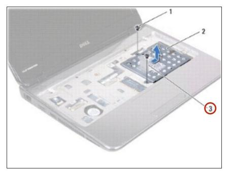
Using the pull-tab, slide the harddrive assembly into the connector on the system board.
