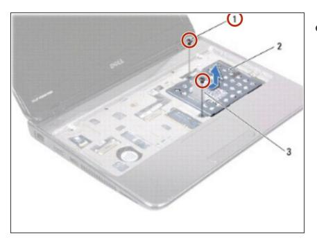
Replace the two screws that secure the hard-drive assembly to the computer base.
