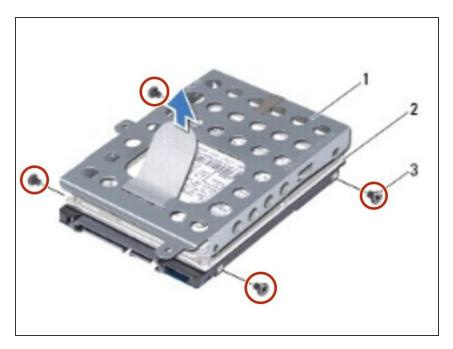
Replace the four screws that secure the hard-drive bracket to the hard drive.
