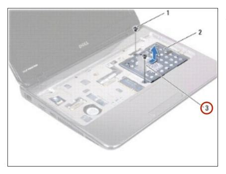
Using the pull-tab, slide the harddrive assembly to the side to disconnect it from the connector on the system board.
