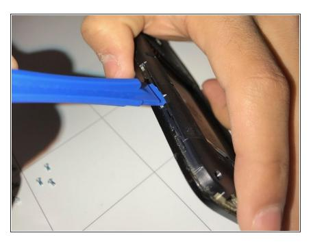
Using your prying tool, place it between the screen and the back cover and pry it open.
