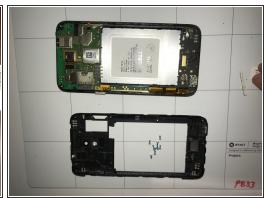
Using the Phillips screw driver, remove the 9 screws from the phone.
