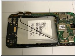
Remove both of this cables located on the bottom left corner of the phone.
