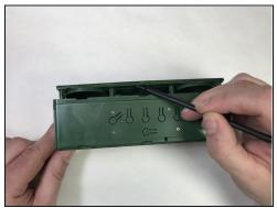
• Using hands or a spudger, pry the front side of the plastic shielding (side opposite of power, control, and auxiliary port cover) from the device.
