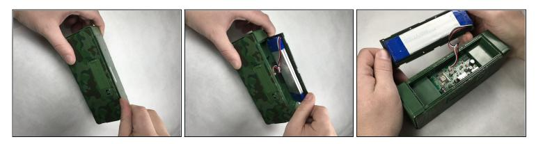
• Using your hands, pry the panel off of the top of the device to reveal the device circuit board and the battery attached to the inner side of the panel.
