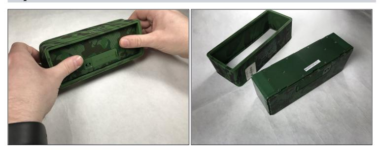
• Turn the device around and gently push the speaker through until it separates from the sleeve.
