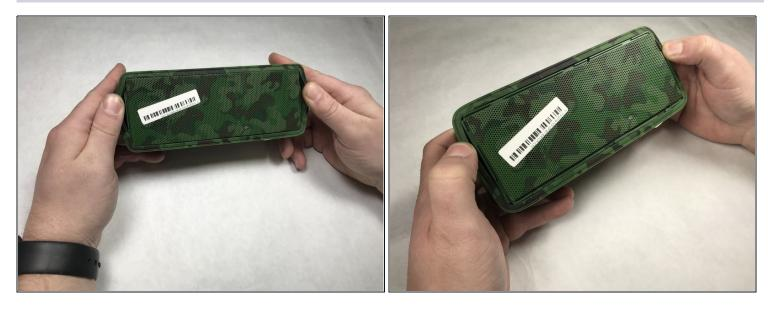
Run your hand around the device where the sleeve connects, lifting lightly up until the edges detach from the device case.
