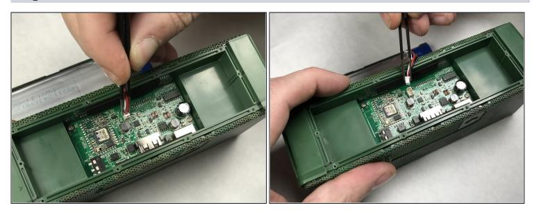
• Using <u>tweezers</u>, carefully detach the battery wire from the circuit board and lift out the panel with the attached battery.
