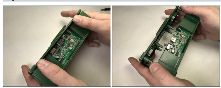
• Turn the device around and remove the rear panel from the device to reveal the device's speaker units.
