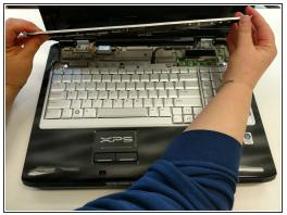
Remove the plastic trim at the base of the screen screen. Start from the tab on the right side and work to the left side.
