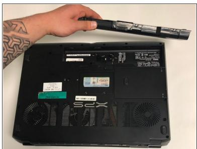
Lift and remove the battery.
