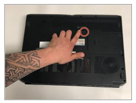
Push the sliding button near the battery compartment.
