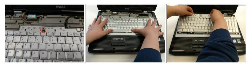
• Remove the keyboard by sliding it forward, off of the clips, and then lifting up.
