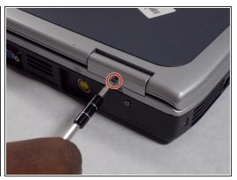
Remove the two 5mm Phillips #0 screws from the hinges
