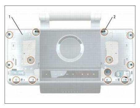
Unscrew the six M2.5 x 5-mm screws on the left side (#1) of the top cover, then unscrew the seven M2.5 x 5-mm screws on the right side (#2) of the top cover.
