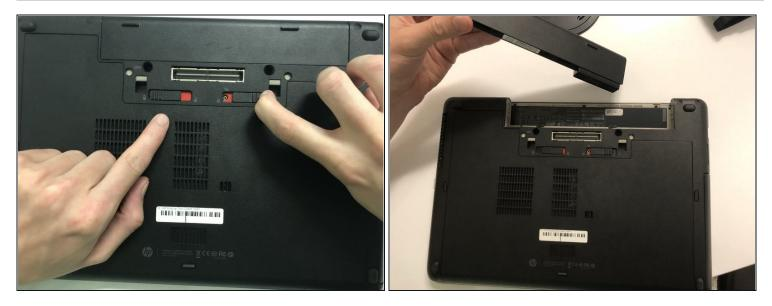
• Pull on both slots outwards as shown in the images to unlock the battery. The battery will not come out if the slots are locked. The battery should easily slide out without much force.
