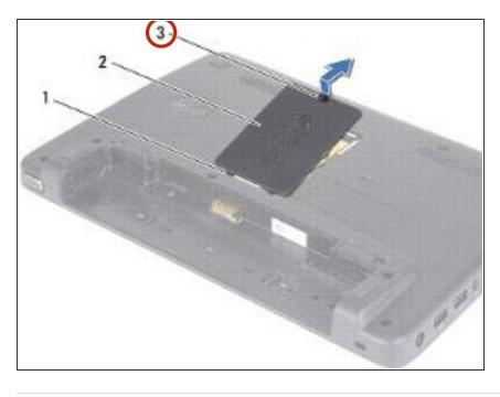
Tighten the screw that secures the memory-module cover to the computer base.
