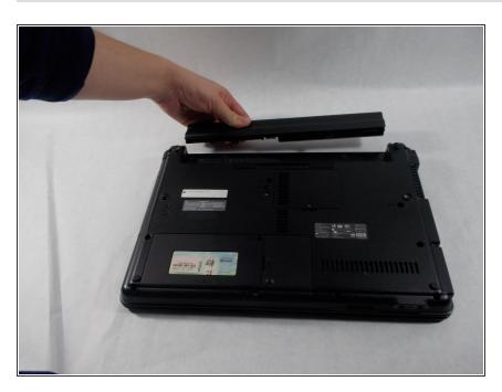
The battery should pop off and release from the device.
