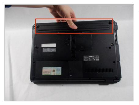
Turn the laptop over, the battery is located along the top of the device.
