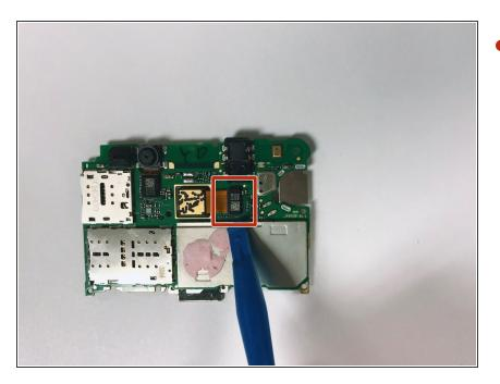
Use a plastic opening tool to pry up and disconnect the camera from the motherboard.
