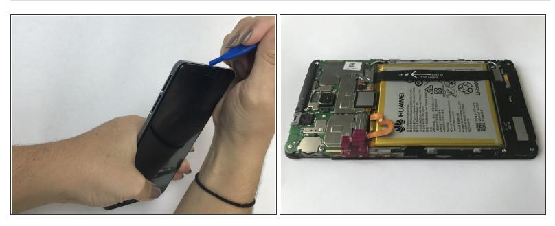
• Pry off the back with a plastic opening tool.
