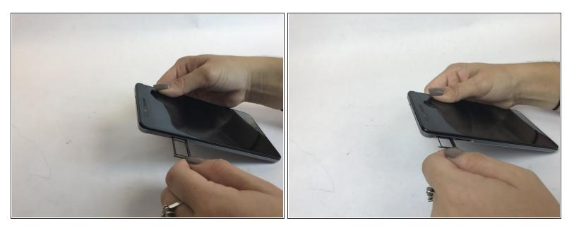
• Use the Sim card ejection tool to remove both the sim card trays.
