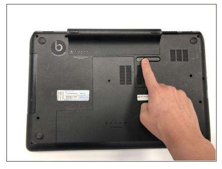
Slide the battery release switch to the left.
