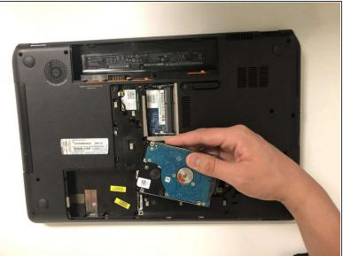
Slide the casing off of the hard drive.
