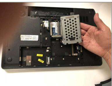
Grab the black tab on the hard drive and pull left and then upwards to remove.
