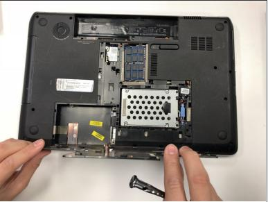
Remove service hatch by sliding away from the computer and lifting up.
