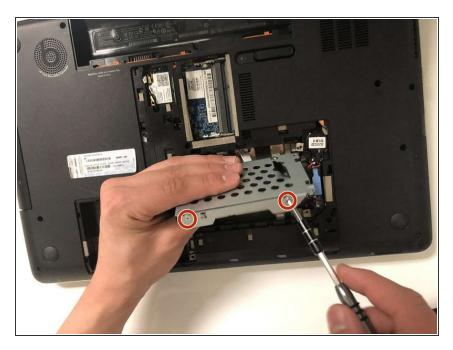
Remove the four Phillips #00 screws holding the hard drive to its case.
