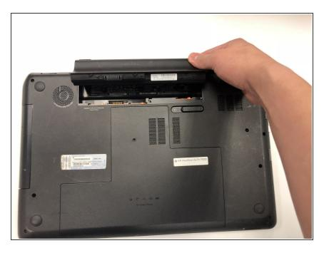
Hold the release switch all of the way to the left and your other hand to pull the battery out.
