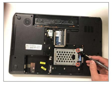
Remove the two Phillips #00 screws holding in the hard drive.
