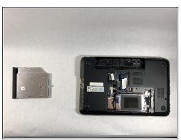
Using a plastic spudger, push the optical drive out toward the left of the device
