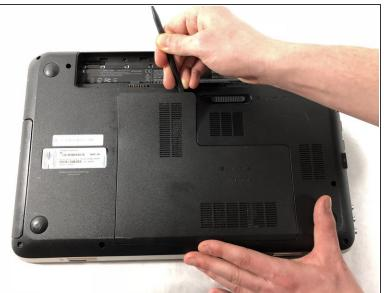
Slide a black spudger under the top of the cover to loosen the clips underneath.
