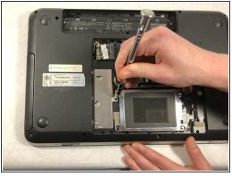
Using a Phillips #0 screw driver, remove the single 4mm screw holding the optical drive in place
