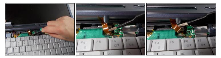
• Use the <u>tweezers</u> to disconnect the ribbon cable from the motherboard.
