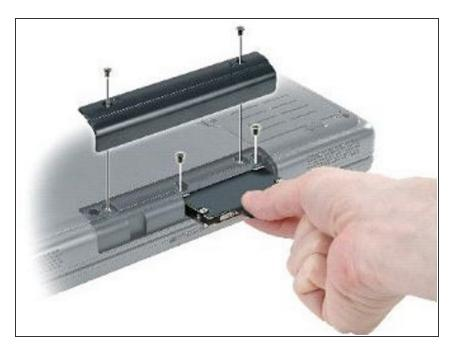
• Lift the hard drive cover and remove the screws used to secure the hard drive.
