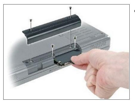
A black plastic strap is attached to the hard drive to assist in removal. Grasp the strap and pull straight out to remove the hard drive from computer.
