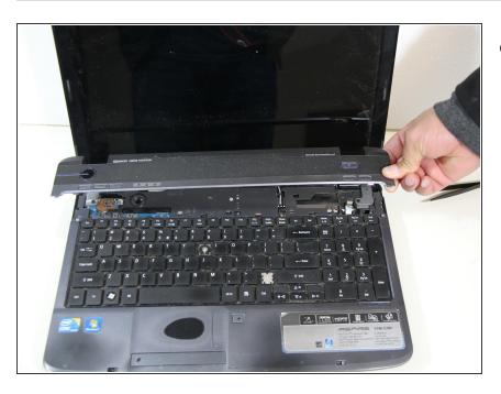
Finally remove the middle cover completely from the computer.
