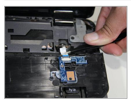
Use tweezers to detach the cable from the volume button board on the middle cover.
