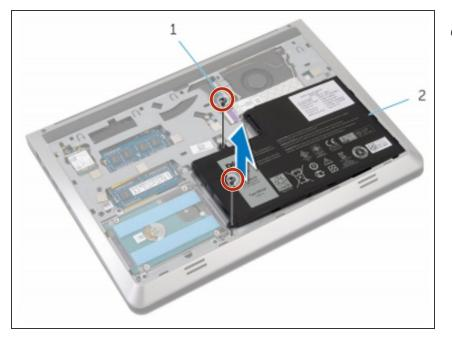
Align the screw holes on the New battery with the screw holes on the base frame and press down on the battery to connect it to the battery connector.
