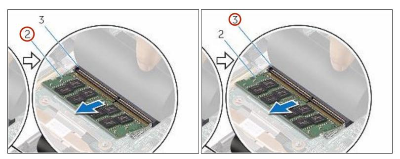
Use your fingertips to carefully spread apart the securing-clips on each end of the memory-module slot until the memory module pops up.
