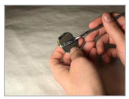
Use a metal spudger to remove the golden retaining clip from the screen. There will be some adhesive to break.
