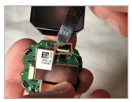
Unhinge the black retaining hinge by prying it open with the metal spudger; Your fingernails will work as well.
