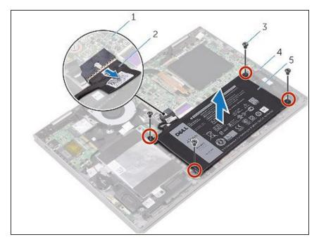
Align the screw holes on the NEW battery with the screw holes on the palm-rest assembly.
