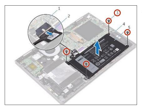
Replace the four screws (M2x3.0) that secure the battery to the palmrest assembly.
