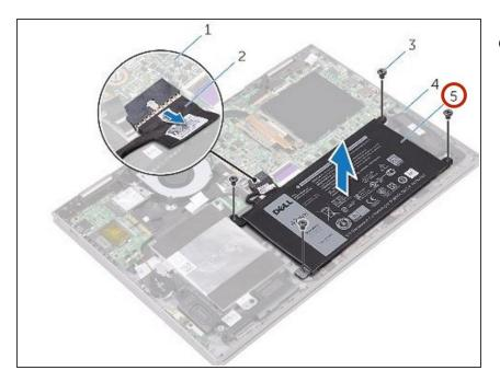
Lift the battery off the palm-rest assembly.
