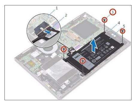
Remove the four screws (M2x3.0) that secure the battery to the palmrest assembly.
