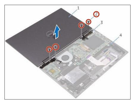
Replace the four screws (M2.5x2.5) that secure the display assembly to the palm-rest assembly.
