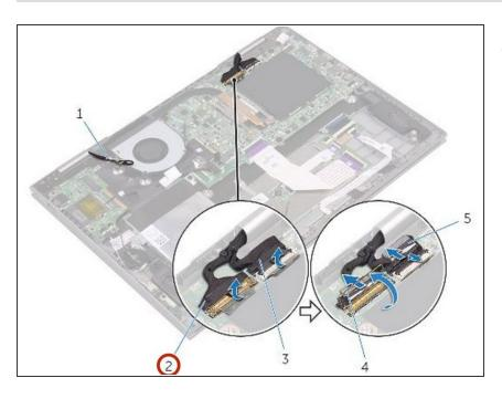
Open the latches to disconnect the display cable and the touch-screen board-cable from the system board.
