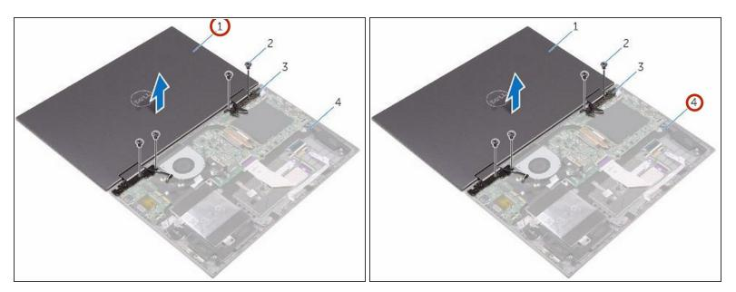
Place the NEW display assembly face down on the palm-rest assembly.
