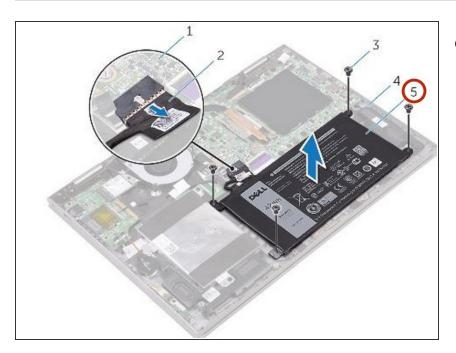
Lift the battery off the palm-rest assembly.
