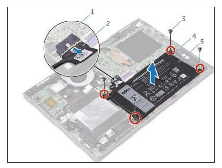
Align the screw holes on the battery with the screw holes on the palmrest assembly.
