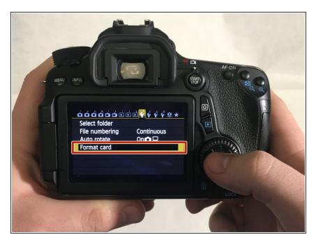
Scroll down the list using the thumb pad and select, "Format card" by pressing the center of the thumb pad labeled, "SET".
