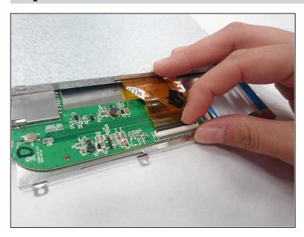
• Unclip JIF clip and remove ribbin cable.
