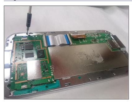
Use a Phillips #00 screwdriver to remove the fifteen 4mm screws from the silver peripheral edging.
