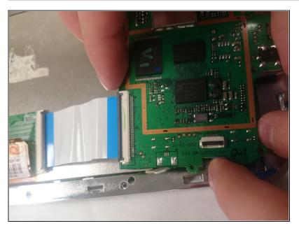
• Unclip ZIF clip from the chip and unplug ribbon cable.
