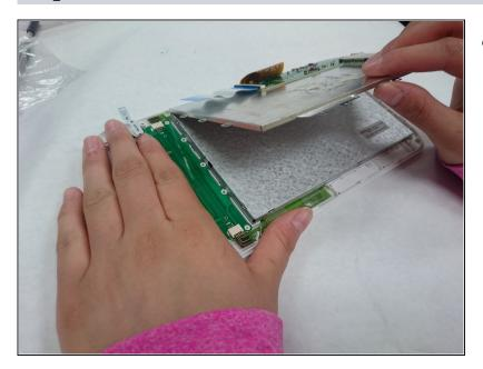
Remove the silver backing plate and the adhered SD port chip.
