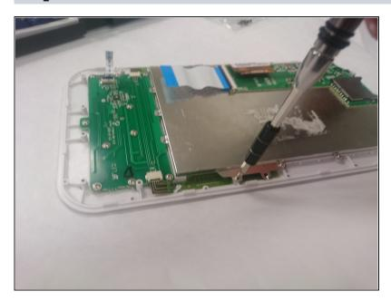
Remove screws from the large metal shielding.
