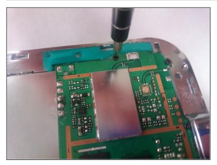
Use a Phillips #00 screwdriver to remove three 4 mm screws from the circuit board containing the headphone jack and power jack.
