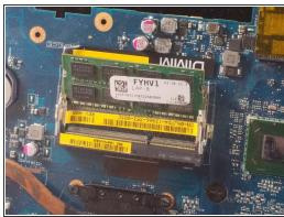
Press the tabs on the RAM inward. The SRAM should pop out of the slot and be easily removed.
