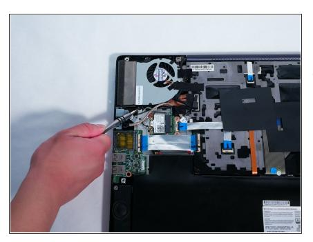
Inspect computer fan for dust accumulation. If dusty, move on to the next step.
