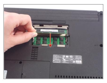
Slide the RAM card out of its socket.
