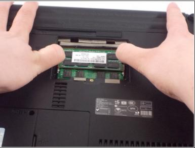
• There are two tabs on either side of the RAM card that are holding it in place. Slide them to the sides; one to the left and the other to the right. The RAM pops out.
