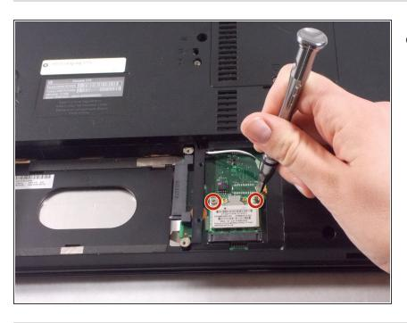
Remove the two .4 cm screws with a PH00 bit.
