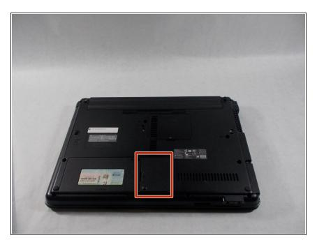
The wireless card is located on the bottom of the laptop, however the hard drive case must be removed in order to access the wireless card.
