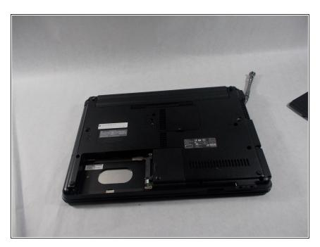
Slide the hard drive case off in a horizontal motion away from the device to remove the hard drive.
