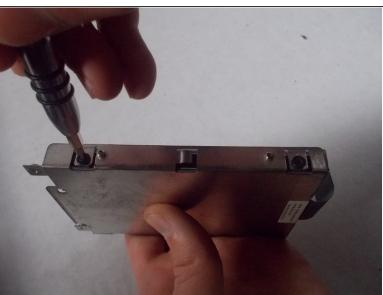
• Remove the four Philips #0 (3mm) screws around the case for the hard drive. There will be two screws and the left and right side.
