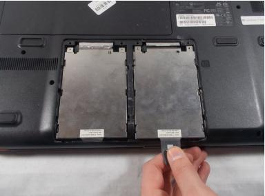
Pull the plastic tab as shown to remove the hard drive from the device.
