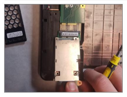
Lift the silver rectangular box up and slide outwards to remove USB Drive.
