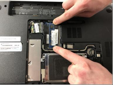
Push the tabs on both sides away from each other to free the RAM, which will raise to a 45° angle.
