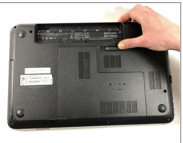
Begin removing the bottom cover by sliding the battery removal slider to the right to pop off the top
