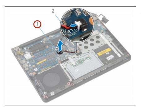
Peel off the coin-cell battery from the system board.
