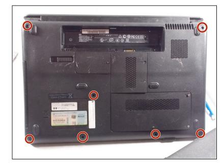
• Remove the seven Phillips #1 screws from the back side of the laptop.
