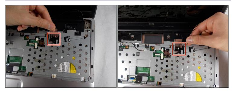
• Remove the black wire from the top right corner by gently pulling outward.
