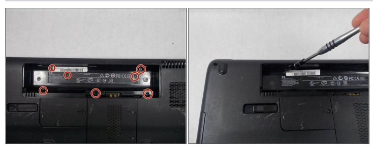
• Remove the seven Phillips #0 screws from the battery compartment.
