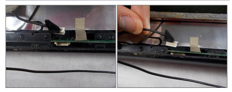
• While the screen is still propped open remove the black wire from the bottom middle of the screen by pulling gently.
