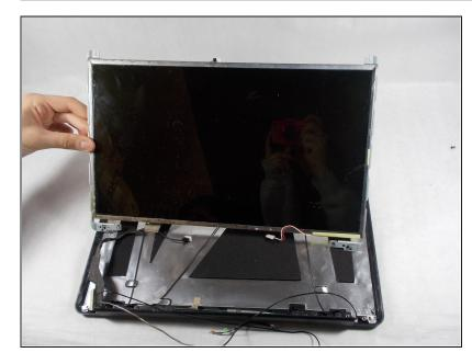
• Remove the screen from the outer casing carefully.
