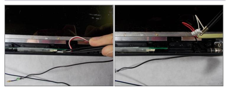
• Using the tweezers remove the red and white wire from the bottom of the screen.
