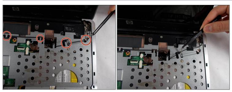
• At the top right of the laptop remove the black wire from under the metal tabs using the <u>tweezers</u>.
