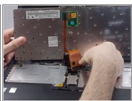
Lift the keyboard and remove the keyboard ribbon cable from the laptop
