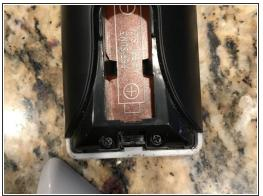
• First off, take off the back and then remove the battery cover. Take out the batteries. Then grab your screwdriver and take out the two screws.
