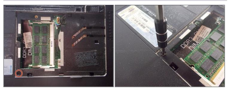
• Unscrew the 2.5x5 mm screw inside the RAM compartment.
