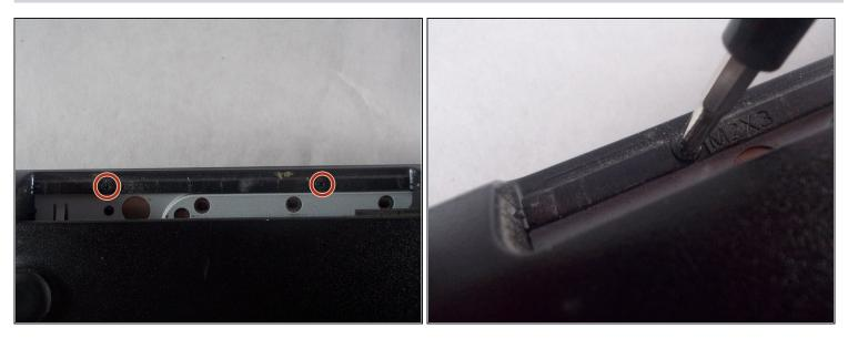
• Unscrew the two 2x3 mm screws inside the disk drive compartment.
