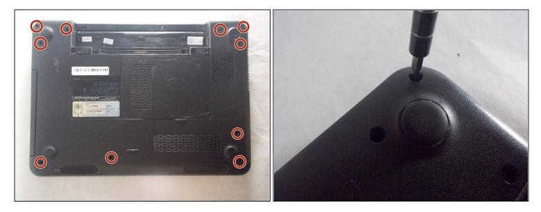
• Remove the 10 2.5x5 mm screws from the base of the laptop.
