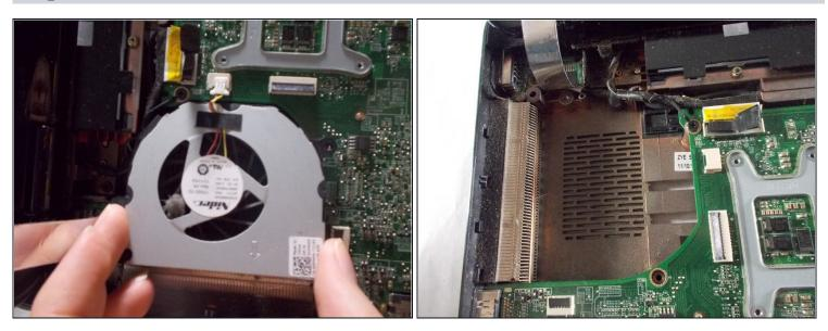
• Pull up and remove the fan from the laptop.
