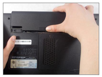
• Push upward from the base of the battery.
