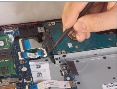
Using a black nylon spudger, disconnect the black connector that attaches the hard drive to the motherboard
