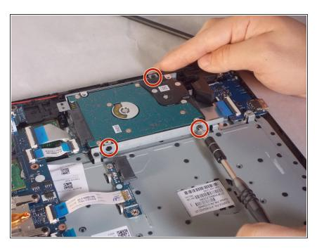
Using the Phillips #0 screwdriver, unscrew the three screws holding the hard drive down to the board.
