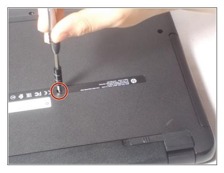
Using the Phillips #0 screwdriver, remove the 7.5mm screw from the underside of the plastic frame that holds the disc tray in place.
