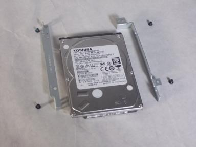
Using the Phillips #0 screwdriver, unscrew the four screws from the holding apparatus.
