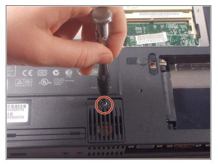
Using a Phillips #1 screwdriver, remove the 4.5 mm screw securing the fan cover to the device.
