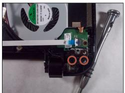
Unscrew the four 6mm screws from each of the laptop hinges using a Philips head #00 screwdriver.
