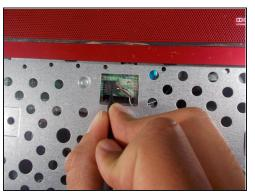
• Remove the wires attached under the keyboard.
