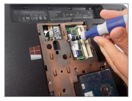
Remove all the screw that secures the keyboard to the computer using a Phillips #0 screwdriver.
