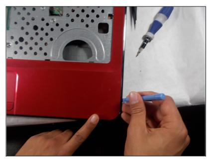
Pry open the bottom of the laptop by using the opening tool to open it up. Do this around the entire outer edge of the laptop.
