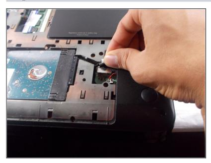
Disconnect the hard drive connector cable from the motherboard.
