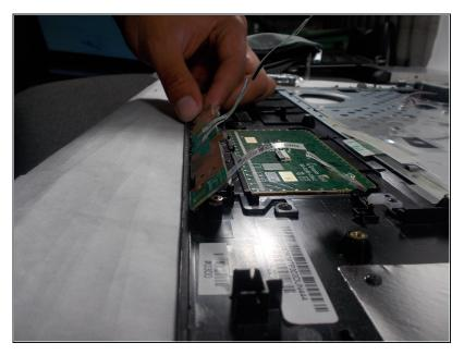
• Carefully lift and remove the button board.
