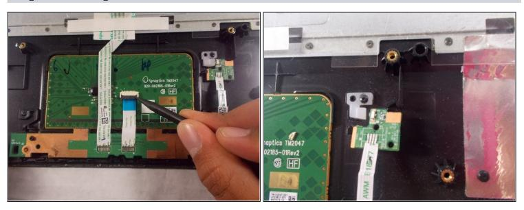
• Remove the wires attached to the button pad.
