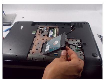
Lift the front edge of the hard drive, then pull the hard drive out gently.
