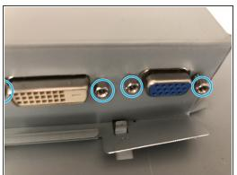
• The First one is connected by four screws in every corner. The second bigger one is connected by 9 hooks like on a picture frame, bend them back to free the cover. For the second one you also have to unscrew the ports for the plugs, screw them to the left to take them off. Once you have lifted the tabs and unscrewed the ports, just lift it off
