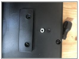
There are 12 screws connecting the back of the monitor and the stand to the front, make sure to keep track of the screws and put them back in the correct spot.
