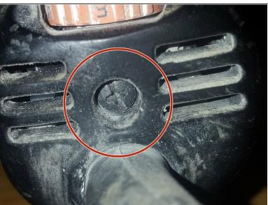
First, remove the single black screw from the end of the handle
