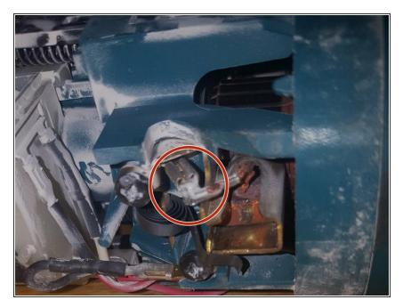
Remove the carbon, and unclip the wires connected to it.
